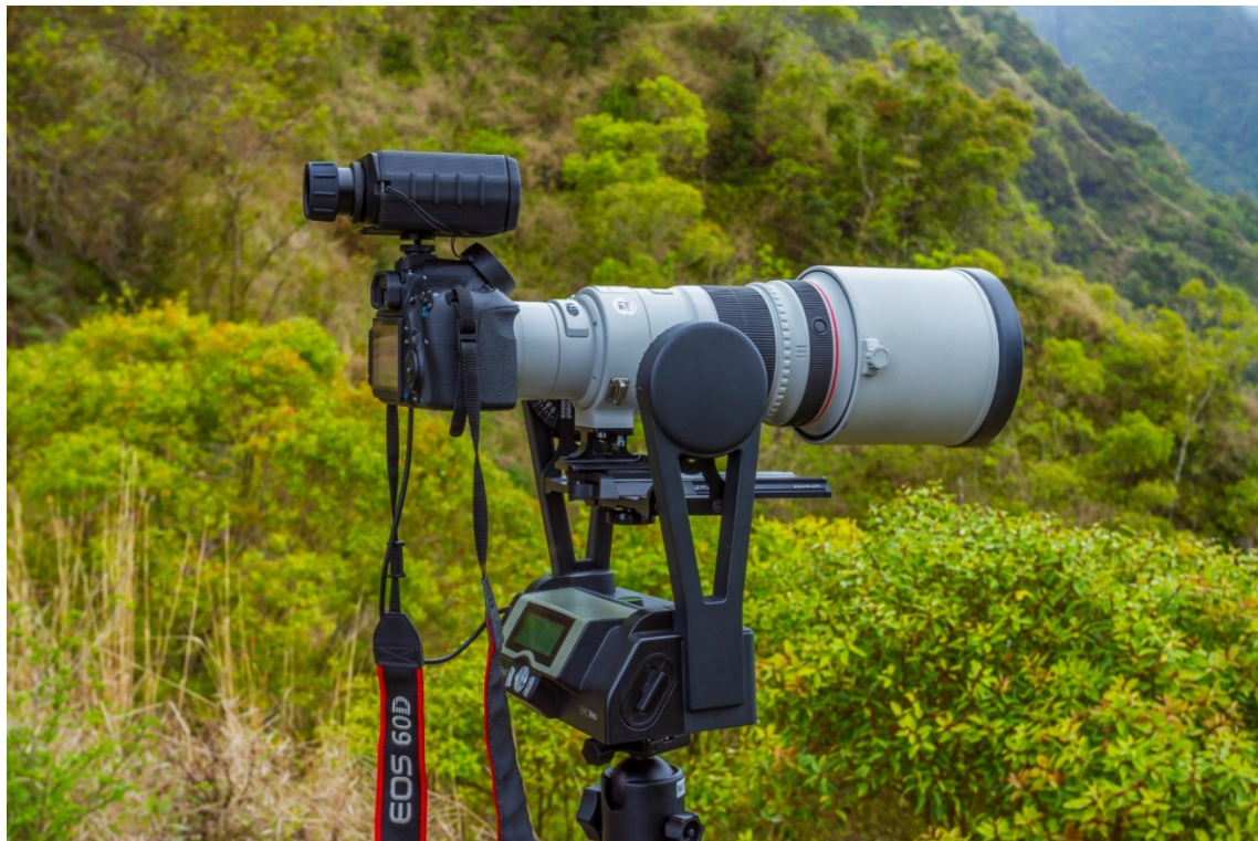
Figure 2. The Gigapan Epic Pro, Canon 60D, and TruePulse 360R rangefinder setup used for image acquisition
